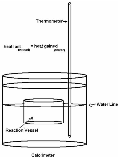
Equation for the calculation of heat is:  $q = mC\Delta T$
